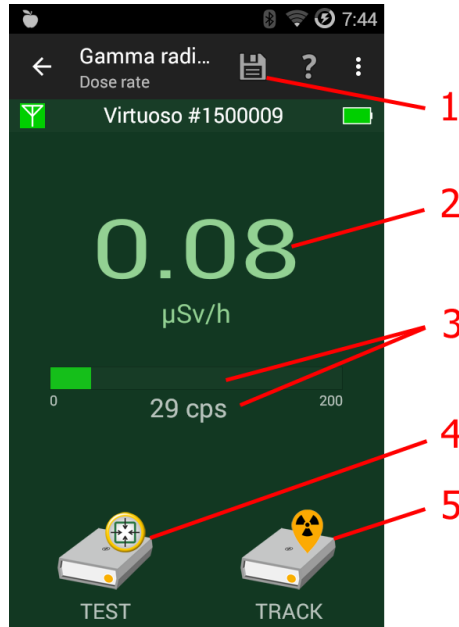
Figure 2.4 - Mode of gamma radiation dose rate measurement
