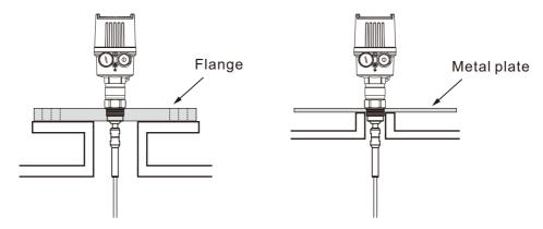
During installation, please avoid using the extension tube on the container. Please install the sensor leveled with the top cover of the container as possible. If this cannot be done, please use a shorter extension tube. Please do not install this instrument at the inlet to ensure that the meter is in a stable position in the medium and not in the inflow position of the liquid to avoid false measurements when the liquid flows in.
