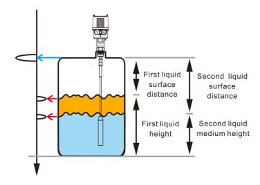
Dual Liquid Level Interface Measuring Condition:
