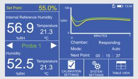
A 4.3" LCD touch-screen runs a powerful UI, which displays all measured values from the reference and probes under test, along with a graphical trend indication of chamber stability. It is also capable of automating complete validation procedures with ease, and providing a complete logged output in csv format straight to your USB memory device, to minimize the time you spend taking readings.
