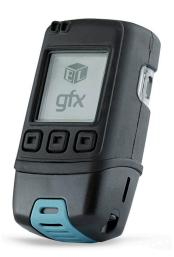
This stand-alone data logger measures and stores over 250,000 temperature and humidity readings over a -30 to  $80^{\circ}$ C (-22 to  $176^{\circ}$ F) and 0 to  $100^{\circ}$ RH range at a resolution of  $0.1^{\circ}$ C ( $0.1^{\circ}$ F) and  $0.1^{\circ}$ RH.
