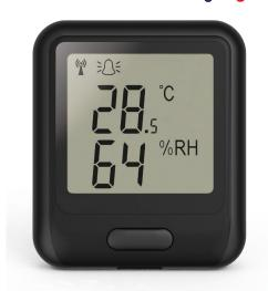
The EL-WiFi-TH+ measures the temperature and humidity of the environment in which it is situated. This high accuracy sensor is typically accurate to ±0.2°C/±0.4°F (+5 to +60°C/+41 to +140°F) and ±1.8%RH (10 to 90%RH @ 25°C). Data is streamed wirelessly over any WiFi network and can be viewed on a PC using free software or on the FilesThruTheAir™ Cloud.
