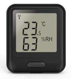
The EL-WiFi-TH measures the temperature and humidity of the environment in which it is situated. This sensor is typically accurate to  $\pm 0.3^{\circ}\text{C}/\pm 0.6^{\circ}\text{F}$  (+5 to  $+60^{\circ}\text{C}/+41$  to  $+140^{\circ}\text{F}$ ) and  $\pm 2.0\%\text{RH}$  (20 to 80%RH @  $25^{\circ}\text{C}$ ). Data is streamed wirelessly over any WiFi network and can be viewed on a PC using free software or on the FilesThruTheAir™ Cloud.
