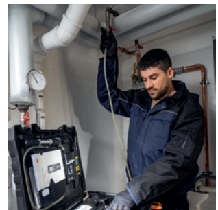
Drinking and waste water test (high-pressure probe up to 25 bar available)
